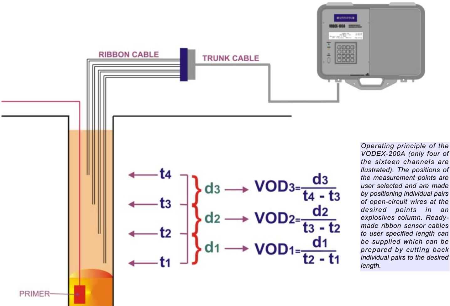
*Operating principle of the VODEX-200A (only four of the sixteen channels are illustrated). The positions of the measurement points are user selected and are made by positioning individual pairs of open-circuit wires at the desired points in an explosives column. Ready-made ribbon sensor cables to user specified length can be supplied which can be prepared by cutting back individual pairs to the desired length.*
